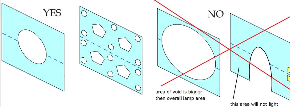
the scribe line, ensure a continuous conductive area is maintained on either side of the scribe line to ensure that all of it lights correctly. Also, the total area of the void should be less than the overall panel area, and symmetry of area should be maintained.
