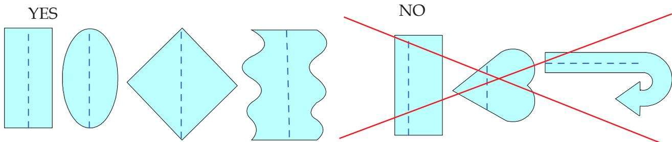
√ The proportion of the lamp area to the scribe length should be close enough to allow adequate electrical conduction and to avoid scribe line heating, uneven luminance, and premature lamp failure.
