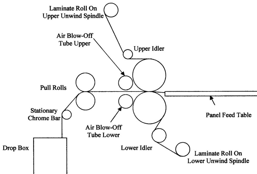
Diagram of a Typical Web Path For Laminating **FLATLITE®** Panel Lamps
